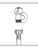
1. Connect the supply pipe by screwing it to a cold water tap using a 3/4 gas threaded connection (see figure). Before performing the connection, allow the water to run freely until it is perfectly clear.
